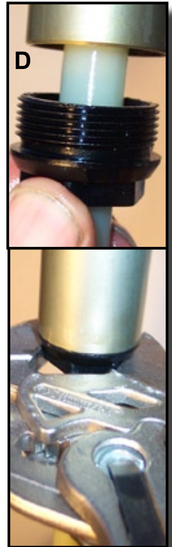
D) Carefully thread in the End Cap and tighten with the flat-jawed pliers.
